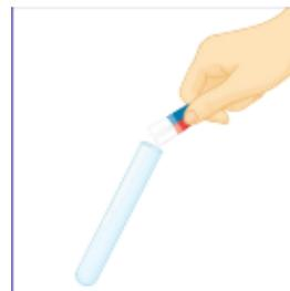
**Test for Chlorine** – **Damp litmus paper** is held over the of gas. If the tube contains chlorine, the litmus paper becomes **bleached** and **turns white**.
