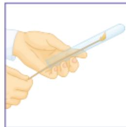
**Test for Oxygen** – Place a **glowing** splint inside a test tube. The splint will **relight** in the presence of oxygen.
